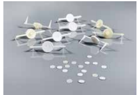
Above: Large and costly quantities of scrap are produced to manufacture micro-sized parts.
